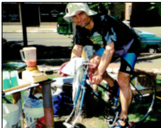
Jan Przysieznik + Bike + magnetic trainer + treadmill motor + blender = pedal powered fruit smoothies
